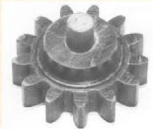
FIGURE 14-2 Single-piece pattern for a pinion gear.
